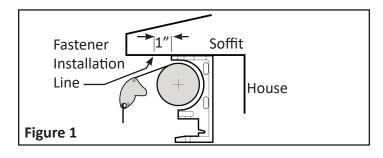
3. Using the marks as a guide, snap a chalk level line along the entire length of the Awning. On the chalk line, mark the location of the **Right End of the Awning**. Along the chalk line, measure 1" further to the right of the Awning end point and a make a mark. This is the location of the first fastener on the right for the Protective Cover.
